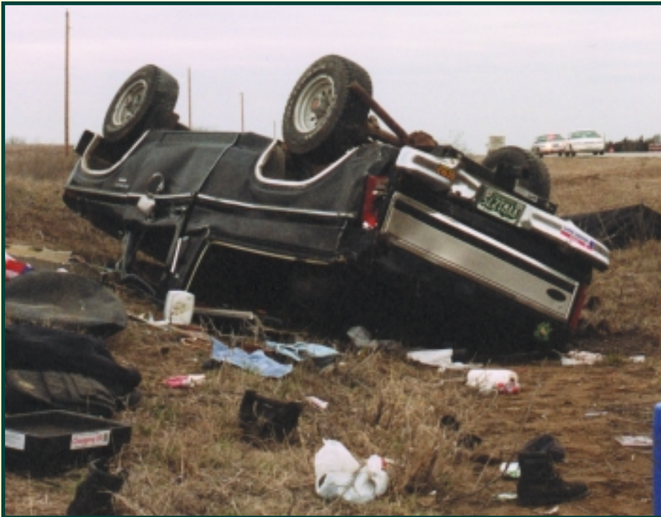
1985 Ford Bronco with separated fiberglass roof.
