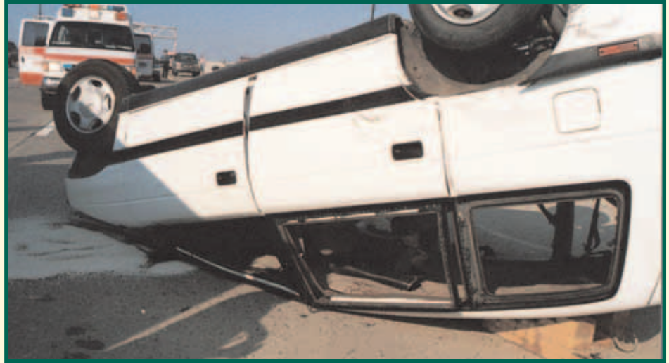
1991 Mazda MPV after tire tread separation.
